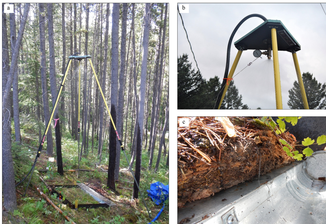
Fig. 3. Photographs of the (a) rainfall simulator extended above the 1 m 2 plot, (b) rainfall simulator nozzle and pressure gauge, and (c) runoff into the trough at the base of the plot showing the metal apron slotted into the organic-mineral soil horizon.
