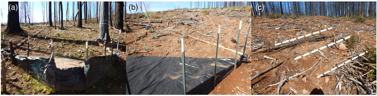
FIGURE 2 Photos of (a) burned-only, (b) salvage logged, and (c) salvage logged and sub-soiled management types. Photos were taken during the second post-fire water year (March 2017). The dashed lines in panel (c) highlight ridges created by sub-soiling that prevented runoff and sediment from reaching fences. We estimated effective area sediment yields in sub-soiled plots based on the plot area from the sediment fence upslope to the first ridge
