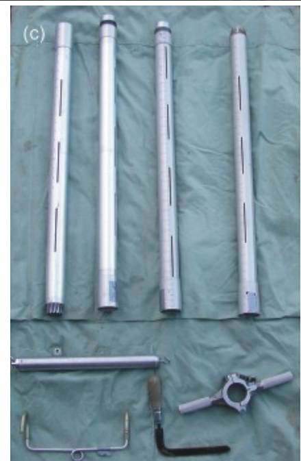
Figure 3. Photograph (a) shows 100- and 33-cm 3 (not used in this study) density cutters; photograph (b) shows 1000- and 250-cm 3 density cutters; and, photograph (c) a Federal snow tube.
