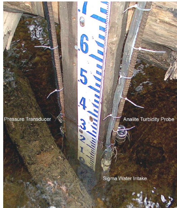
FIGURE 17.3 An example of a suspended sediment monitoring station (under low flow conditions). The probes are mounted on rebar, which is secured at the bottom by placing it into a section of open-bottomed copper pipe. The top of the rebar is bent to 90° and inserted into a hole in the 2 × 6" board. This arrangement keeps the instruments secure during peak flow events, but also allows them to be easily removed for servicing. (Photo: P. Marquis)
