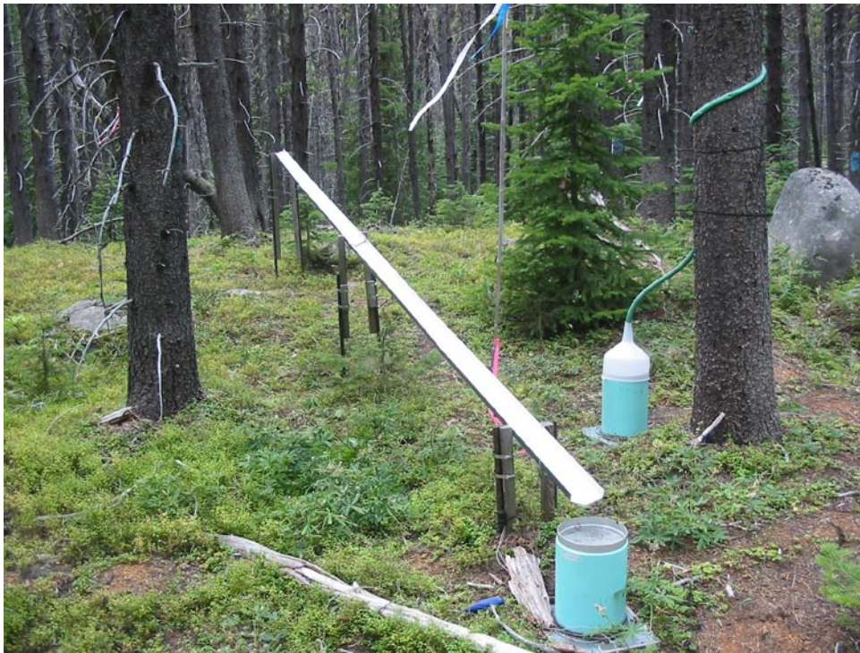
FIGURE 17.2 Long throughfall trough collector emptying into a tipping-bucket rain gauge, Upper Penticton Creek Watershed Experiment, near Penticton, B.C. (Photo: D.E. Carlyle-Moses)
