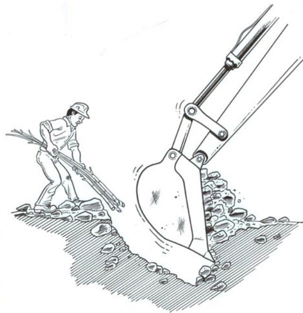
FIGURE 18.34 Live gravel bar staking can be used to initiate natural successional processes on gravel bars that form from excess sediment accumulation associated with development-related landslides or erosion. (Image: D. Polster)
