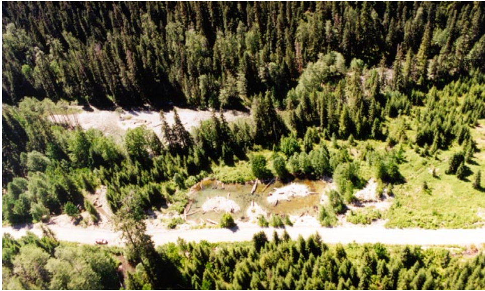
FIGURE 18.54 Off-channel habitat created in groundwater-fed gravel pit and connected to Taylor River, south-central Vancouver Island. (Site work by M. Wright; photo: G. Horel)
