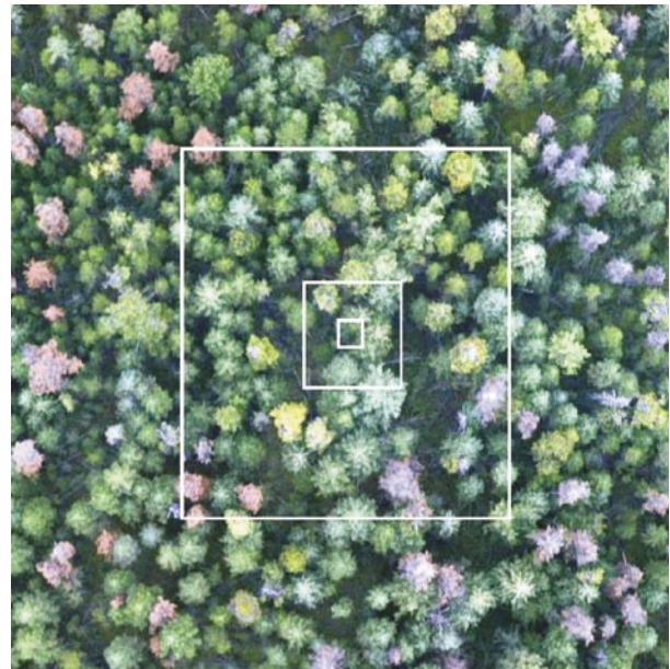
FIGURE 17.8 Illustration of spatial resolution and subsequent information content of three common image spatial resolutions: 30 \times 30 m, 10 \times 10 m, and 2.5 \times 2.5 m. The underlying image is a digital photograph. Image provided courtesy of J. Heath, Terrasaurus Ltd., Vancouver, B.C. Figure adapted from Wulder et al. (2006).
