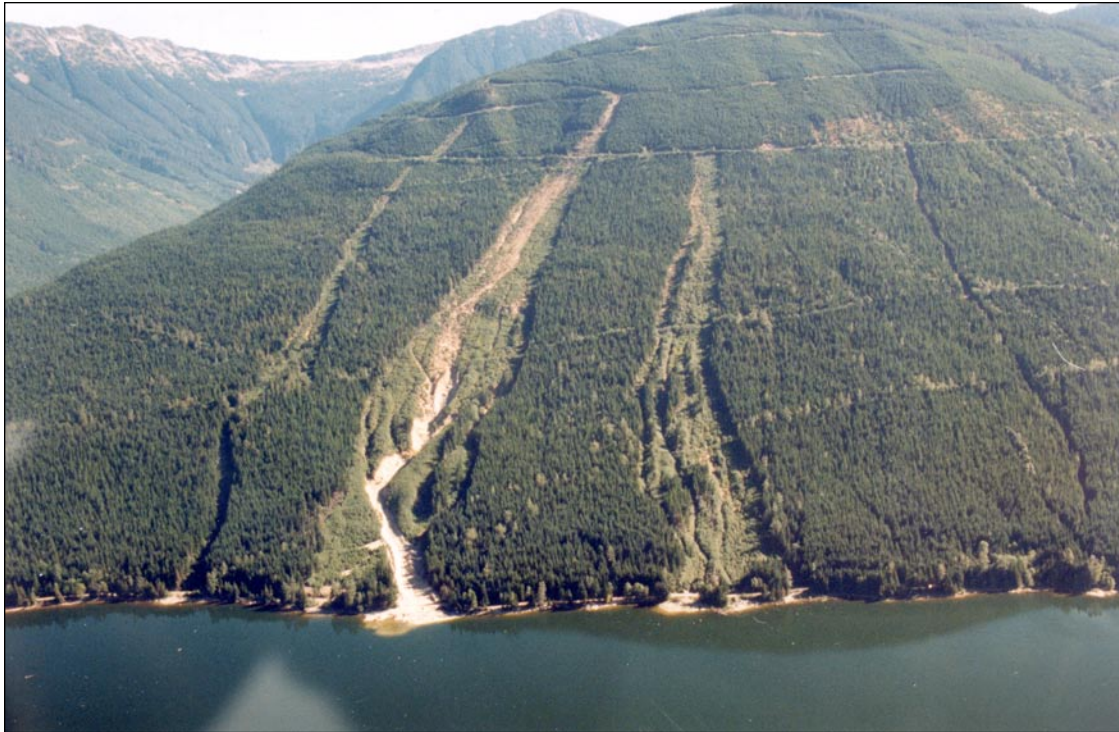
FIGURE 18.9 An example of landslides caused by logging road development. (Photo: M. Miles)
