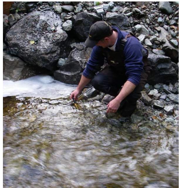
FIGURE 12.5 Measuring stream temperature in a British Columbia coastal stream. (Photo: T. Redding)
