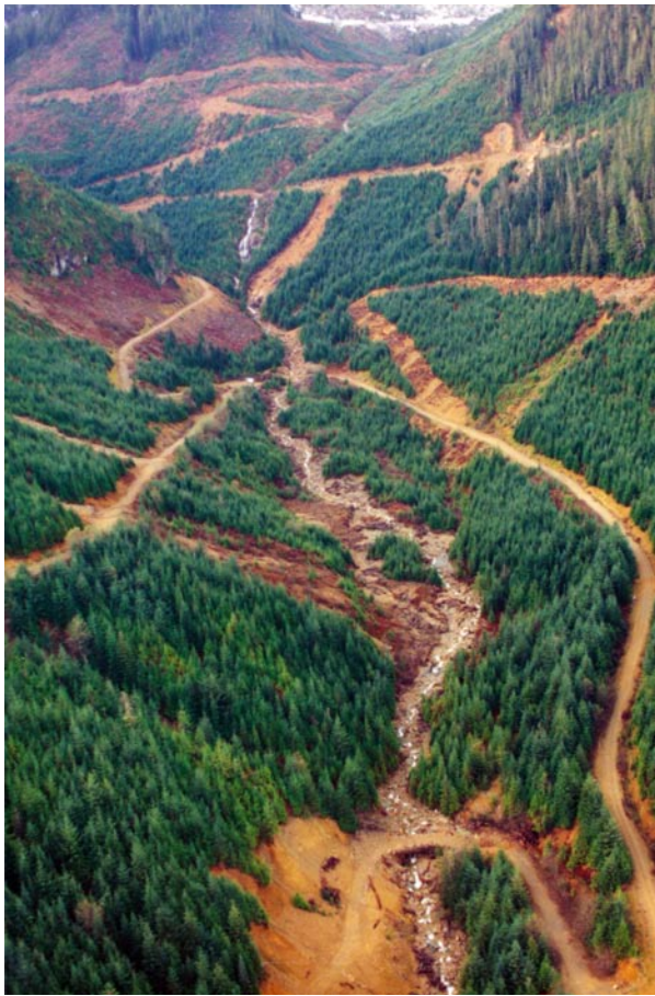
FIGURE 18.5 Misery Creek in the mid-Coast Mountains of British Columbia illustrates landslide and erosion problems that can occur from road construction on steep, unstable terrain. (Photo: M. Miles)
