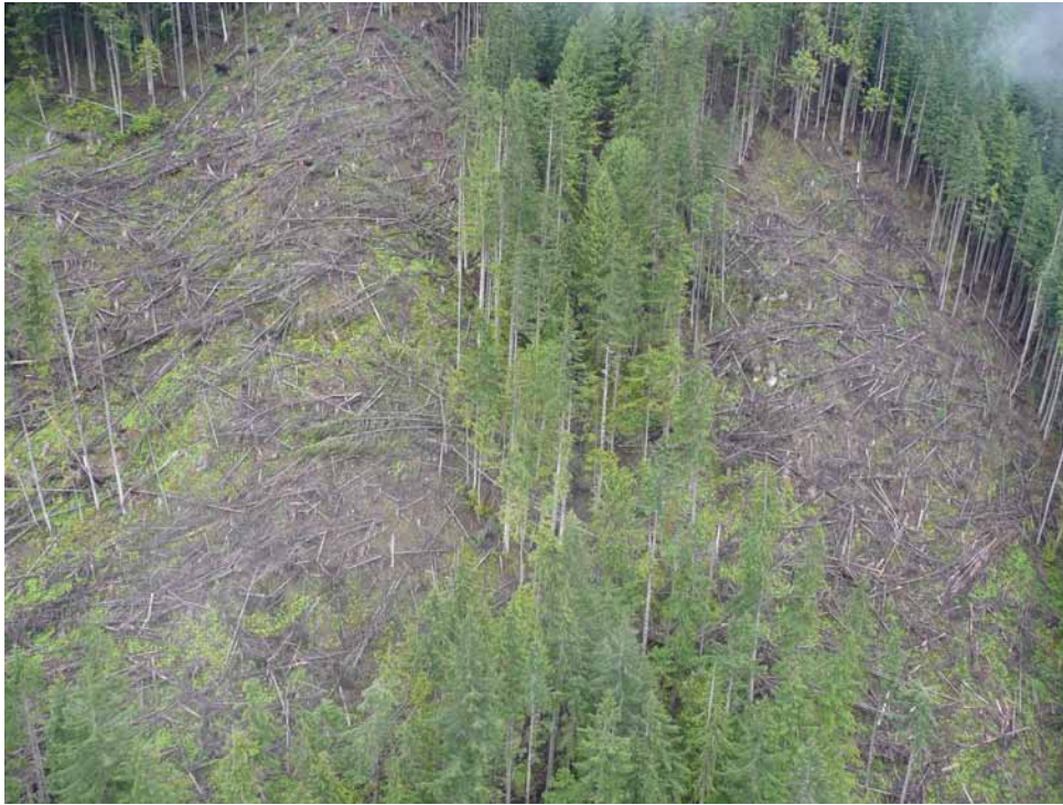
FIGURE 9.35 Small helicopter-yarded patch cuts, with a buffered gully (middle of the photo), at Foley Creek watershed, Chilliwack Forest District. This approach to harvesting near unstable terrain is becoming more common. (Photo: T. Millard)
