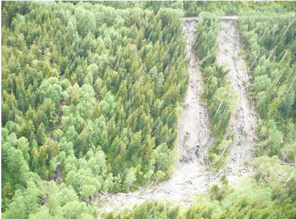
FIGURE 9.16 Two road-fill slope slides associated with uncontrolled road drainage in the San Juan watershed, South Island Forest District. (Photo: T. Millard)
