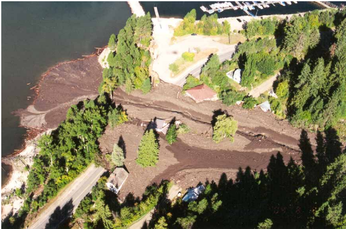
FIGURE 8.48 Debris flow deposit on Kuskonook Creek fan. (Photo: P. Jordan)
