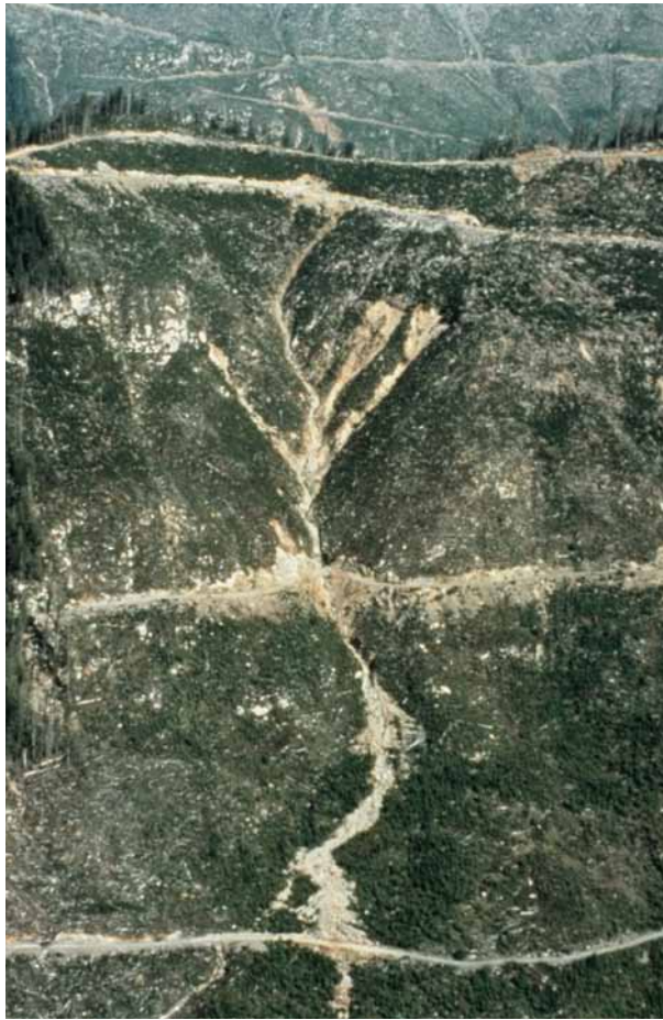
FIGURE 1.4 Example of the effects of pre-1980s harvesting and road-building practices in unstable/erodible terrain, coastal British Columbia. (Photo: B.C. Ministry of Forests and Range)
