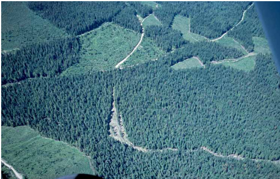
FIGURE 9.13 Debris slide/avalanche that progressed to a large debris flow below a culvert in the Fortynine Creek area of the Kootenay Lake Forest District, 1996. Water flow to the culvert increased because of the cumulative effects of roads and cutblocks over a 20-year period, although culverts, ditches, and road maintenance generally followed accepted standards. (Photo: P. Jordan)
