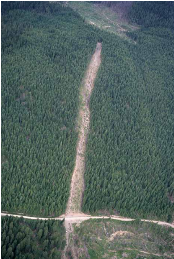
FIGURE 9.19 "Gentle-over-steep" debris avalanche caused by drainage diversions on road and skid trails near Ferguson Creek in the Arrow Forest District, about 1990. (Photo: P. Jordan)
