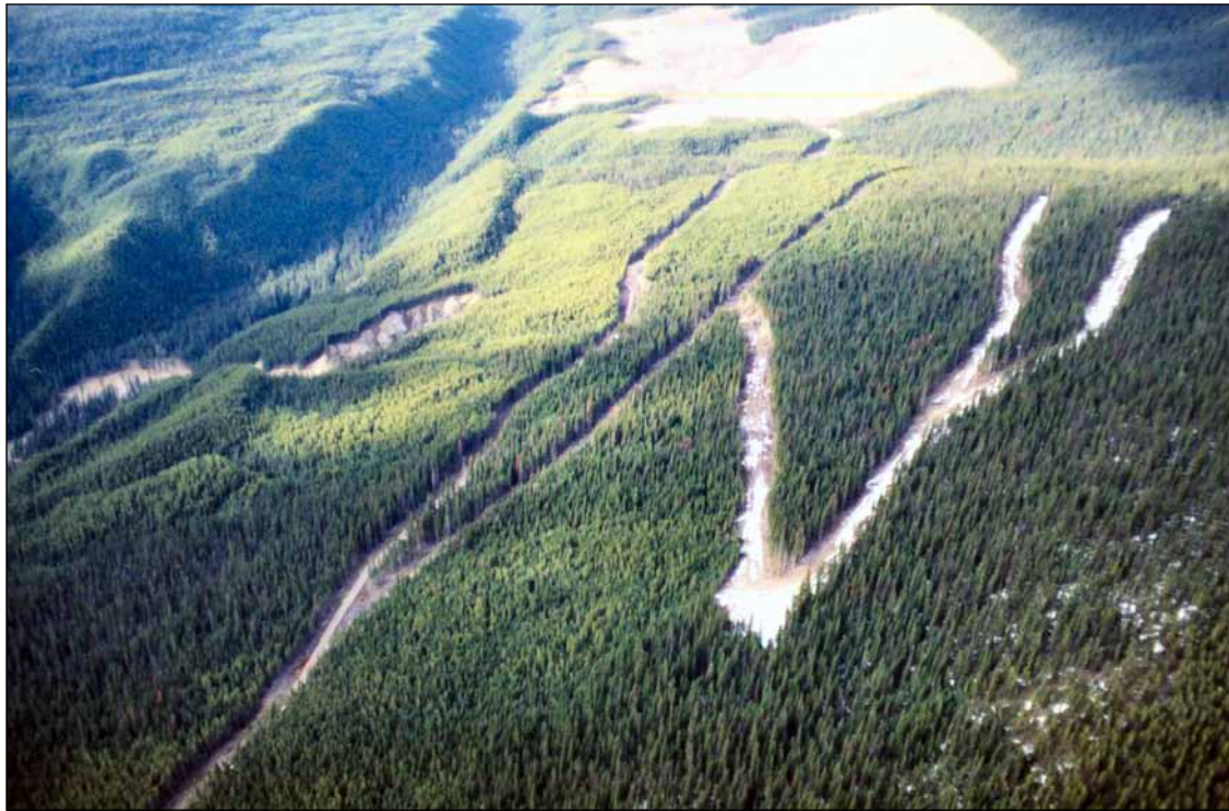
FIGURE 9.24 Natural flow pathways downslope (right to left in photo) are intersected by roads on the hillslope above Donna Creek (far left). (Photo: J. Schwab)
