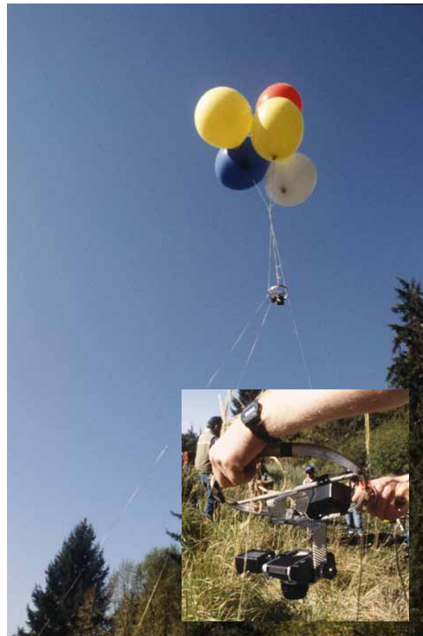
FIGURE 1.8 Demonstration of low-level aerial photography using helium-filled balloons to quantify changes in stream channels at Carnation Creek, 1989. (Photos: D. Toews)
