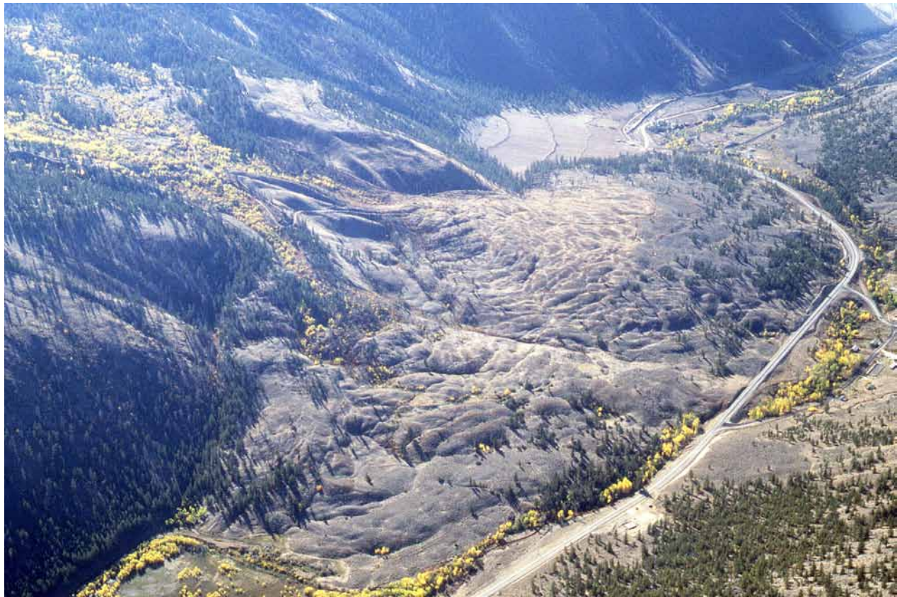
FIGURE 8.28 Pavilion earth flow; note the transverse ridges in the zone of accumulation. (Photo: J. Ryder)
