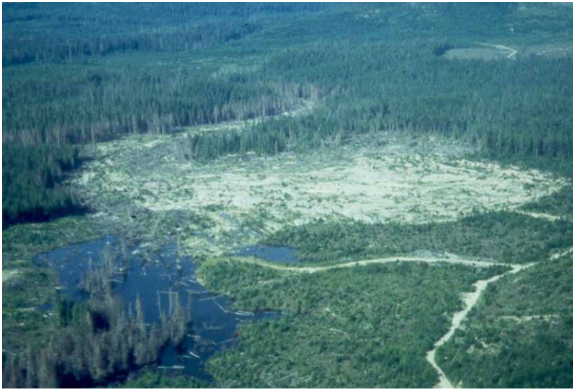
FIGURE 8.26 The Mink Creek earth flow spread illustrates a rapid failure on a nearly flat gradient. (Photo: M. Geertsema)
