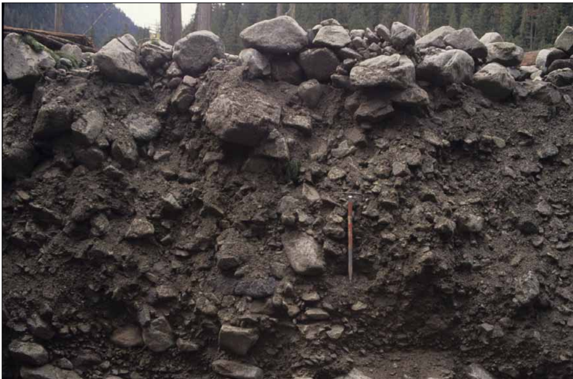
FIGURE 8.24 Debris flow deposit showing inverse grading (larger stones toward top) and matrix support (stones not touching, surrounded by fine material) at Meager Creek near Pemberton. (Photo: P. Jordan)
