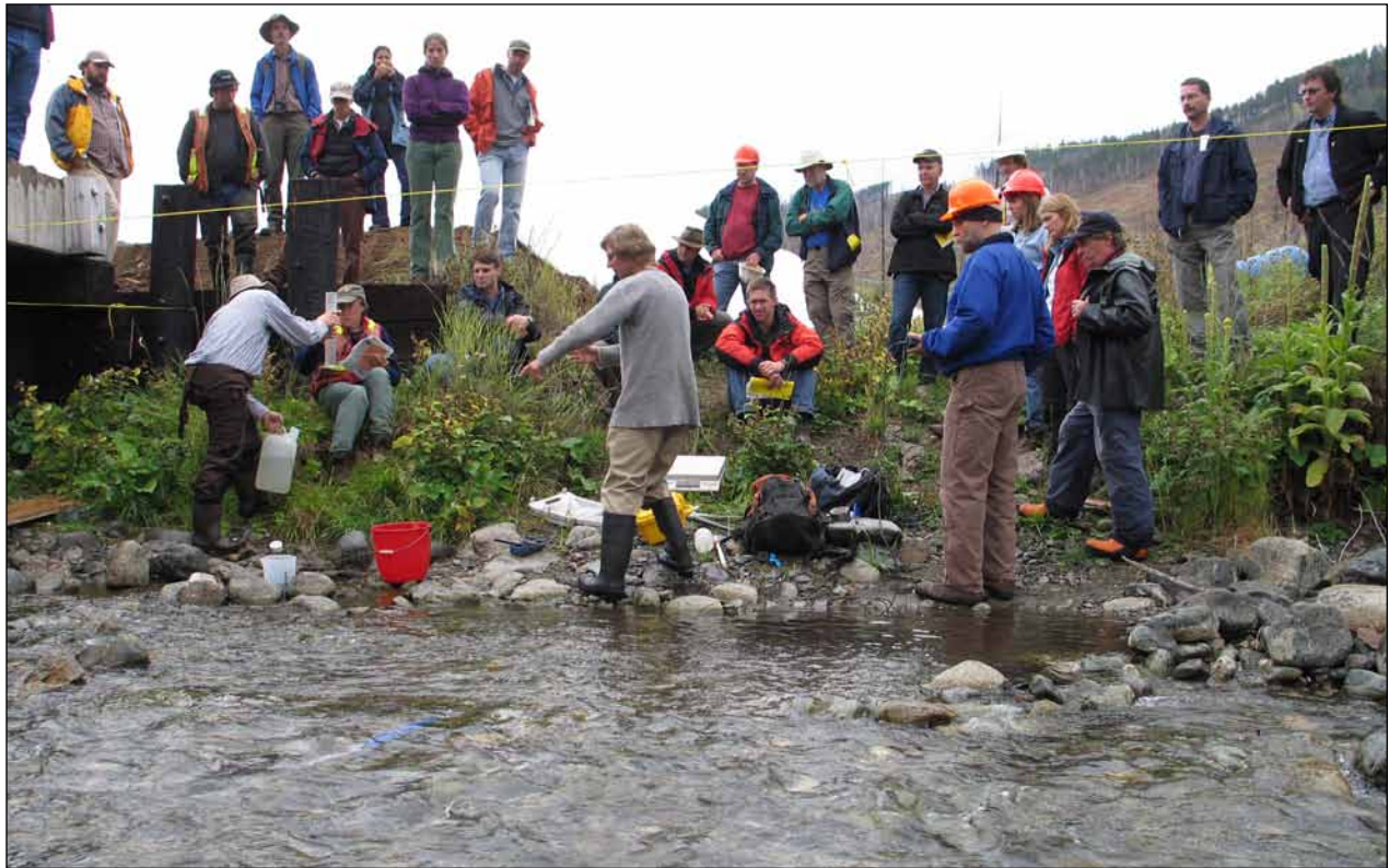
FIGURE 1.6 Demonstration of salt dilution gauging to measure streamflow in Fishtrap Creek, Friends of Forest Hydrology workshop, September 2005. (Photo: K. Turner)
