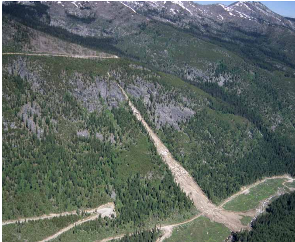
FIGURE 9.18 “Gentle-over-steep” debris avalanche below road and ground-based harvesting near Shaw Creek in the Kootenay Lake Forest District, 1996. In this case, the road and skid trails were properly deactivated, and there were no drainage diversions observed; subtle changes to slope hydrology may have been responsible. (Photo: P. Jordan)
